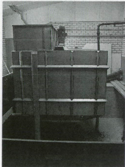
STAINLESS STEEL PREMIXING TANK WITH ELECTRONIC WEIGHING SYSTEM, CONTENTS: 10 M 3
